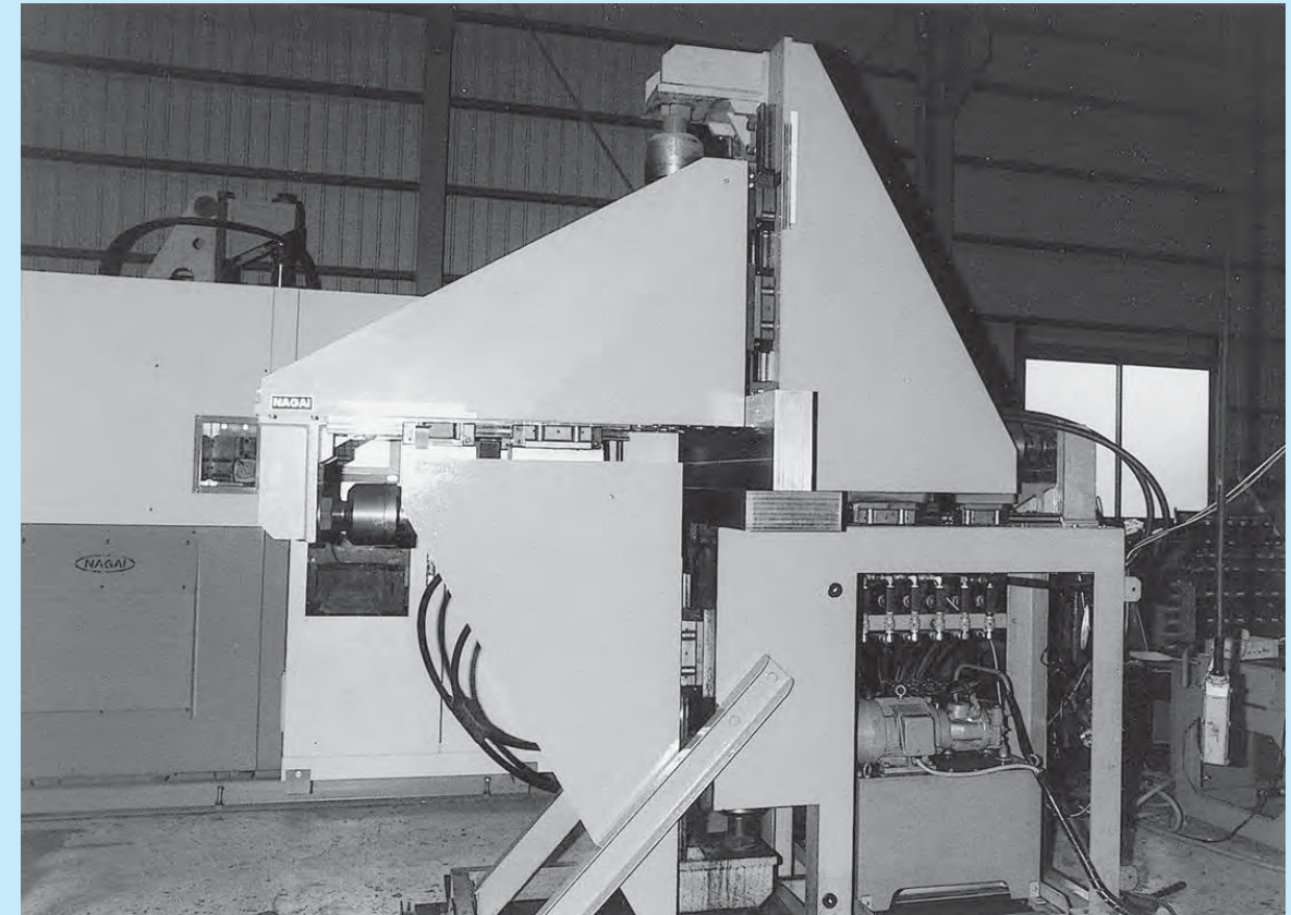
High-pressure high-density lumber compression system
