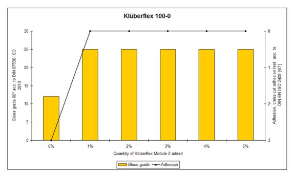
NOTE: The values shown were determined on an EPDM Shore 65 substrate and serve for orientation only. They are no absolute values.
